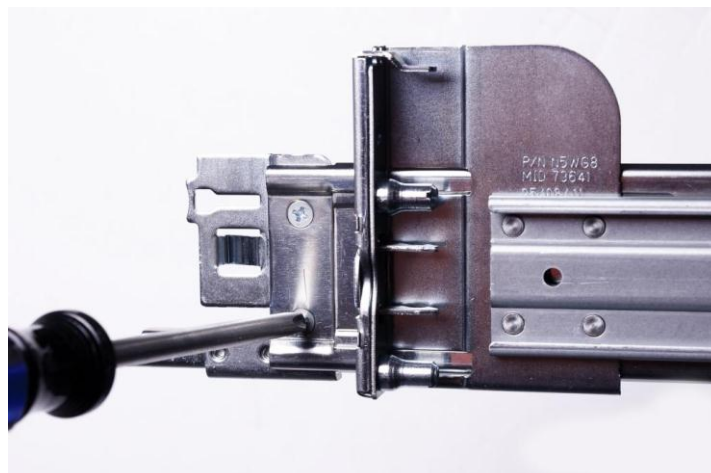
Figure 10. Removing the outer CMA brackets for shallow racks
