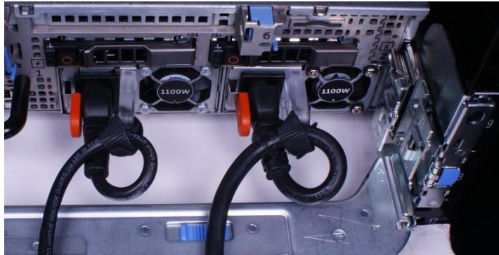
Figure 2. Routing power cables through the strain reliefs
